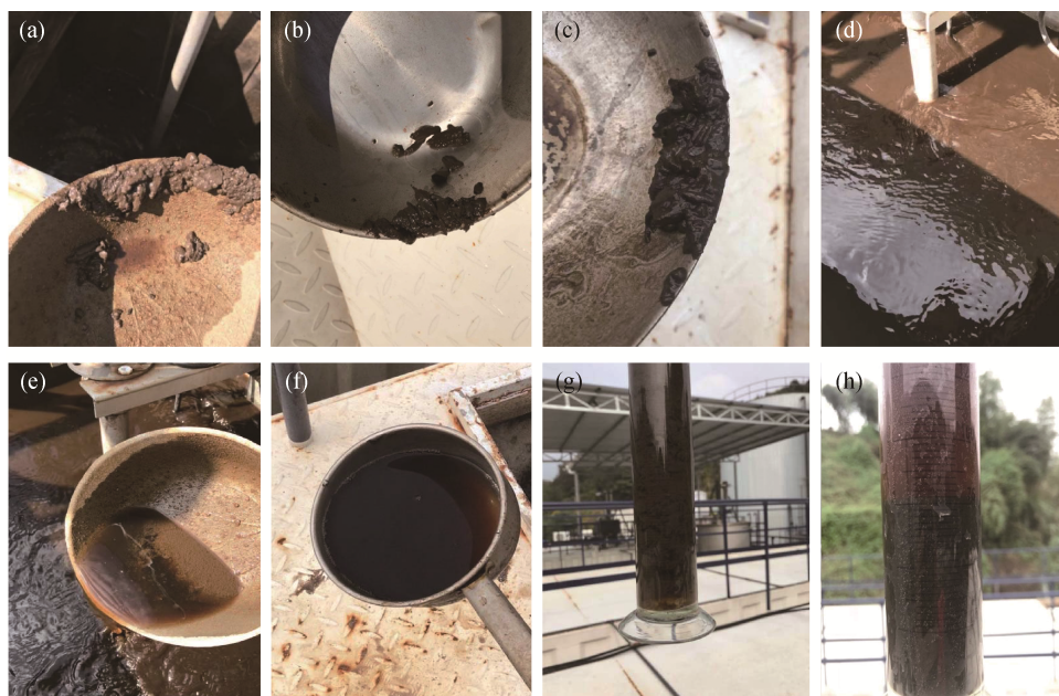
图9 水解酸化池污泥、UASB的出水和底泥以及O池泥水分离状况 Fig. 9 Waste water and sludge in hydrolytic acidification tank, UASB and aerobic tank
