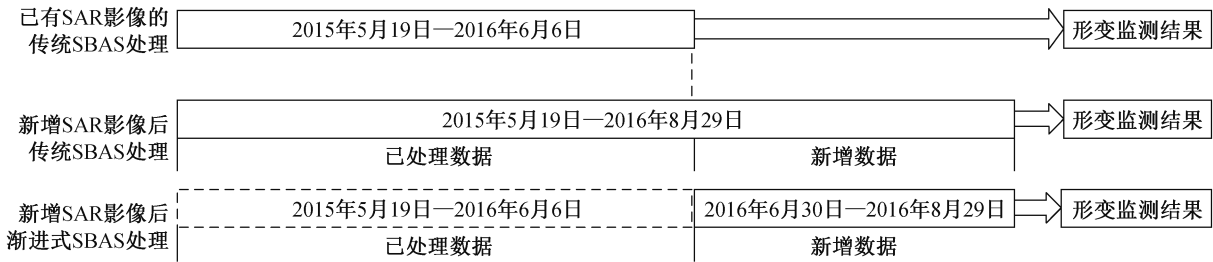
图 4 新增影像后渐进式 SBAS 和传统 SBAS 获取新时刻地表形变的实验设计 Fig. 4 Experimental design of the progressive SBAS and the traditional SBAS method for obtaining surface deformation when new images are added
