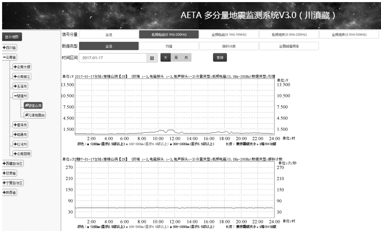
图 3 多分量地震监测系统网页数据查看界面 Fig. 3 Data view interface of multi-component seismic monitoring system's website
